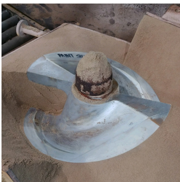
Top, bottom, and mid-section of a stiff extrusion auger sand mold before pouring
