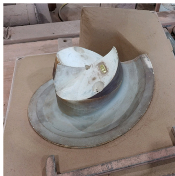
Top, bottom, and mid-section of a stiff extrusion auger sand mold before pouring
