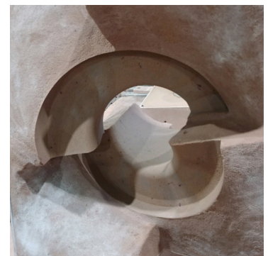
Top, bottom, and mid-section of a stiff extrusion auger sand mold before pouring
