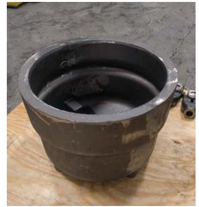
The final product: a hydrant end cap made of iron after casting.
