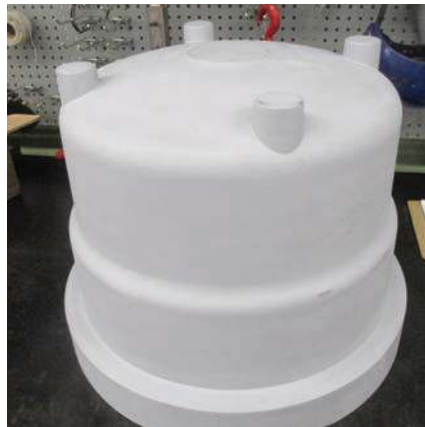
A 3D printed hydrant end cap ready prepared for sand encasement.
